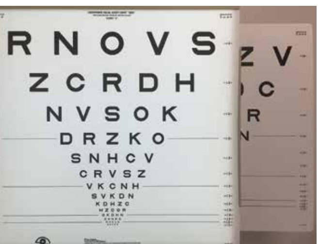
FIGURE 4. Shows the standard backlit ETDRS chart, which sits on a floor stand or wall mounted unit. One of the other alternate charts is shown slightly pulled out on the right side. There are three total charts, one for the right eye, one for the left eye and one for both eyes.
