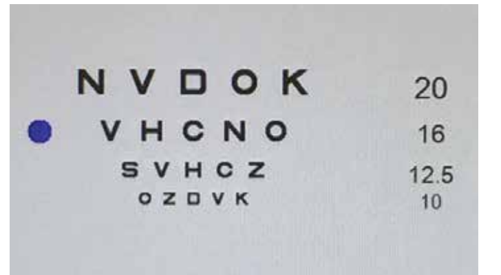
FIGURE 7. Shows the computer screen at 4M after the button for the 20/20 line had been pressed on the tablet. The blue indicator helps the patient zero in on the next line for more detailed testing.
